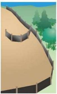
Use J-hooks to trap and pond muddy runoff flowing along uphill side of silt fence. Turn ends of silt fence toward the uphill side to prevent bypassing. Use multiple J-hooks every 50 to 150 feet for heavier flows.
