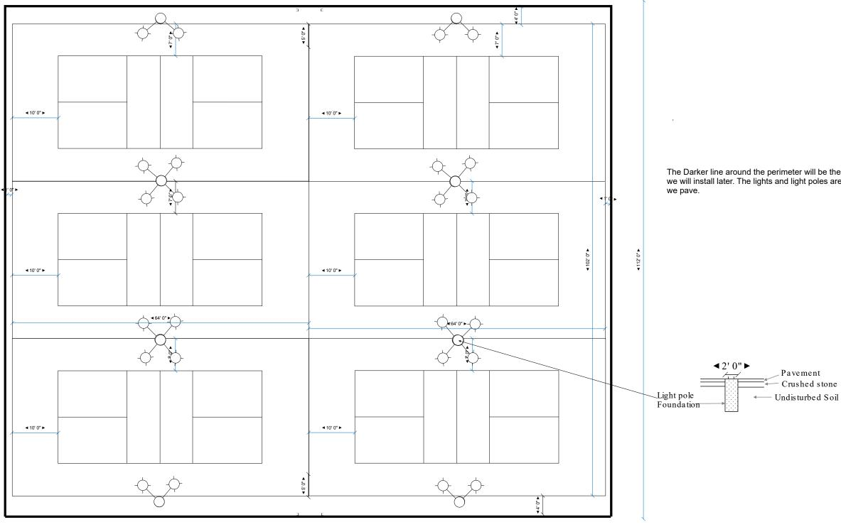
The Darker line around the perimeter will be the the outside of paving, the other lines will be the court markings that we will install later. The lights and light poles are shown in this drawing, but only the footings will be installed when we pave.
