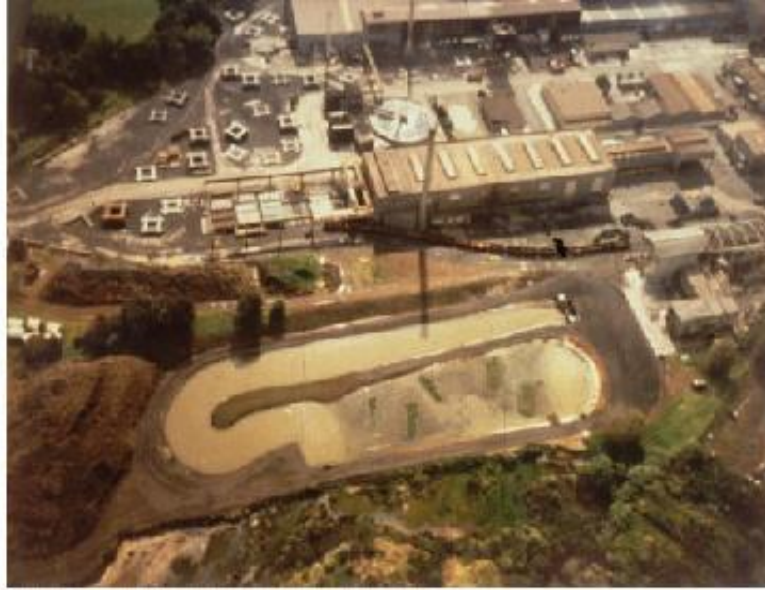
Figure PTP-03- 10 Pond/Wetland System
